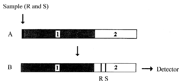
Fig. 1. Schematic illustration of the partial filling technique (PFT). (A) Sample introduction in a capillary partially filled with the chiral selector (zone 1). (B) After separation, the resolved enantiomers migrate through the zone without selector (zone 2) towards the detector.
